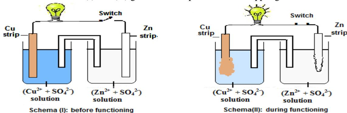
1- Describe the construction of the galvanic cell represented by schema (I).
